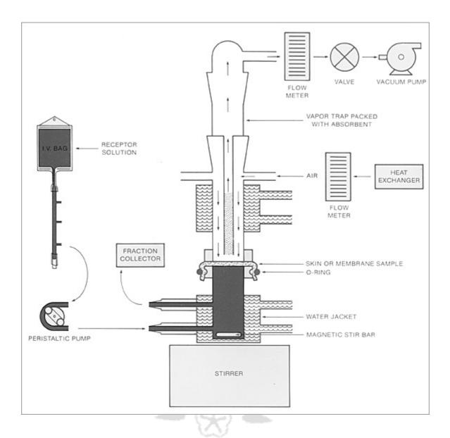
The above diagram shows how a typical penetration/evaporation system is set up. A sample of the membrane or excised skin is placed over the penetration cell, dermal side down, and is held in place with an o-ring. After the topical preparation is applied to the surface of the skin or membrane, an evaporation cell is clamped over it.
