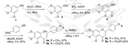
With chalcones **4** in hand, intramolecular oxidative cyclization of chalcones **4** to flavones **5** was accomplished in DMSO solution at refluxing temperature catalyzed by catalytic amount of iodine for 30 min in excellent yields (81-93%).
