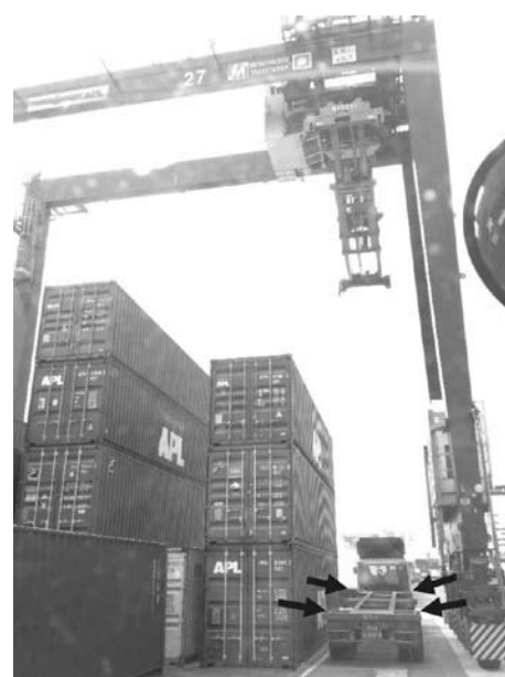
Fig. 1. The overhead crane sets the container onto the unloaded container truck. The driver has to stay in the truck to cooperate with the crane operator to move the truck forward/backward. The arrows mark the pins at the four corners, which have to be inserted into (aligned with) the four recesses of the container.
