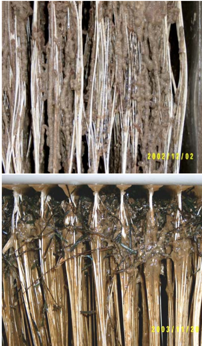
Fig.2 The biofilm on the hollow fibers in SMBR wastewater treatment plant
