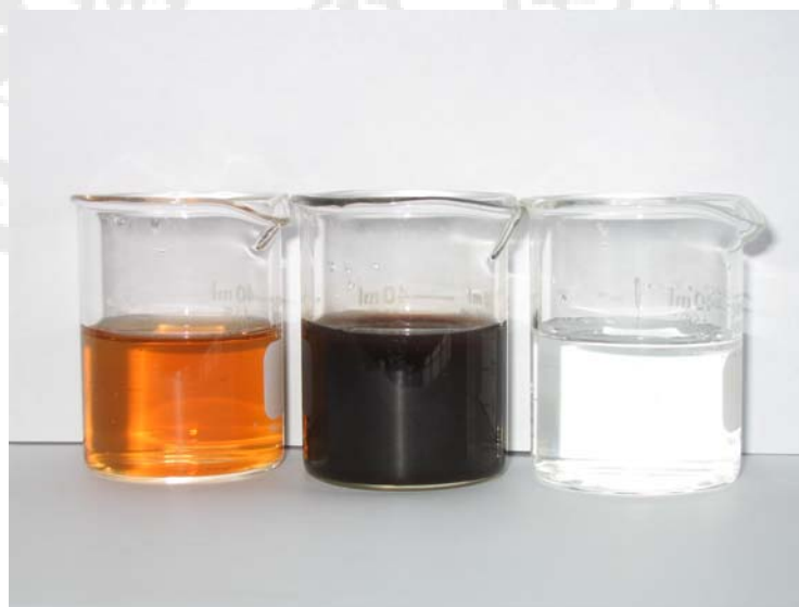
Figure B.6 Aniline solution from the right hand, aniline solution before treatment; the middle, aniline solution after treatment (no filtrated); the left hand, aniline solution after treatment (filtrated)
