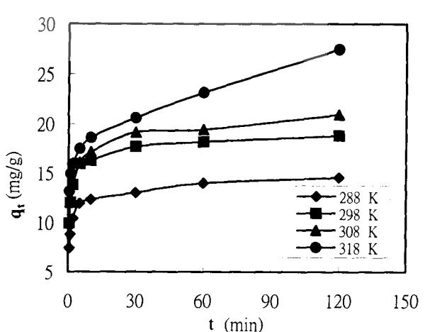
**Fig. 3.** Plots of  $q_t$  vs.  $t$  for adsorption of paraquat on clay adsorbent (RBE-2) at various temperatures.
